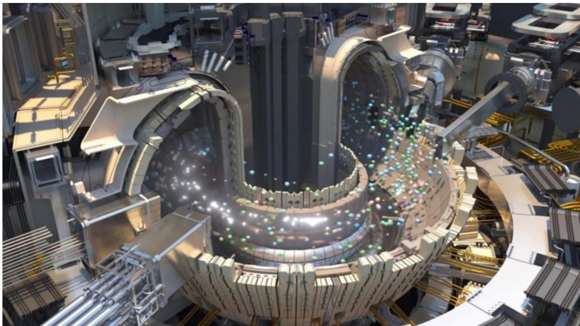
Figure 1 - ITER Tokamak section view showing the internal surface of the Vacuum Vessel protected from the burning plasma by the 440 Blankets modules
